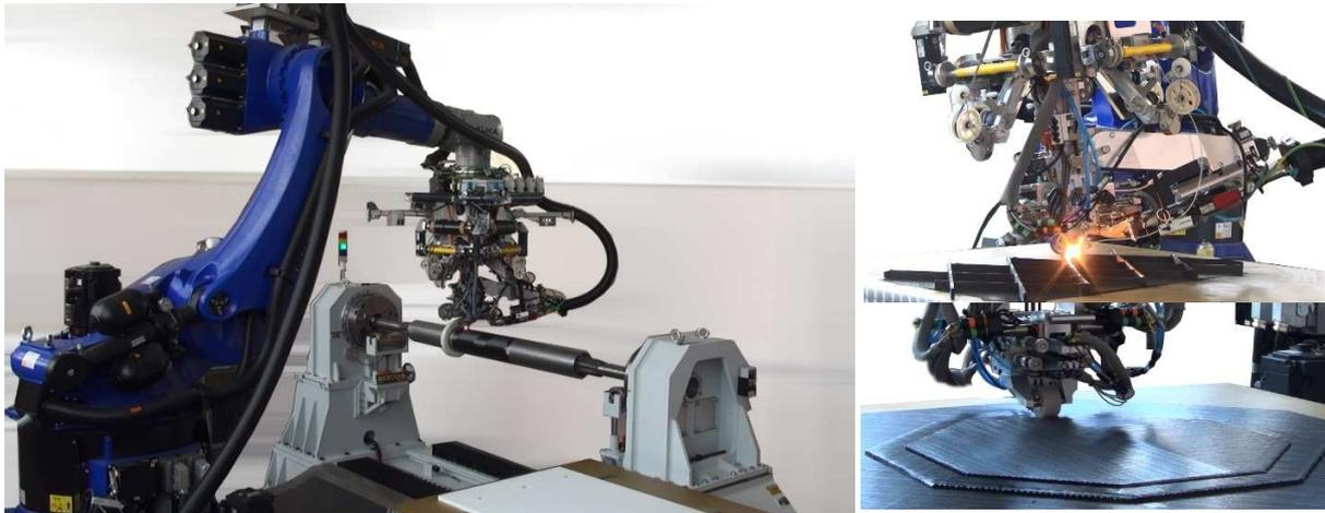
***The multi-material AFP Robot machine performing placement of thermoplastic prepreg***
